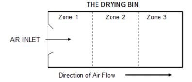
As air enters, the grain in the region nearest the air inlet dries first. This dried zone will move through the grain mass in the same direction as the airflow as drying proceeds.
